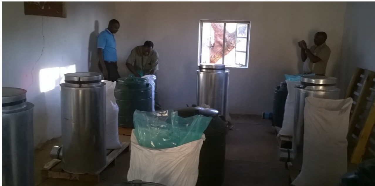
Figure 34: Metal silo for storage of produce using hermetic technology
